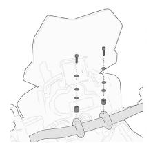
05SKITK Specific kit to mounting the KS900A Smart Bar
